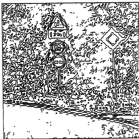
Fig. 3. Edge segmentation performed by the HSC on a 256 \times 256 window
